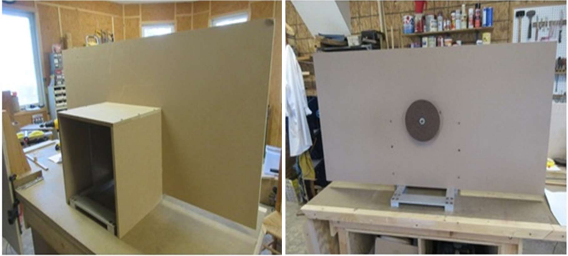
Figure 3. Views of the apparatus within its enclosure. Left panel: view from the participant's perspective. A box-like cover encloses the framework, leaving open the end through which participants insert their hands. The opposite end of the enclosure is a vertical sheet (125 cm wide x 64 cm high) that occludes the disk stimuli as well as the actions of the experimenter from the view of the participant. Right panel: view from the experimenter's perspective.
